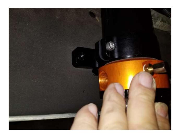
2. Find a suitable location for the fuel pump assembly and mark the two (2) holes using the billet aluminum mounting bracket as a guide.
